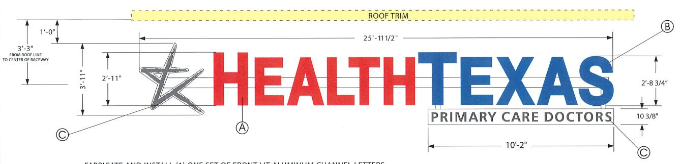
FABRICATE AND INSTALL (1) ONE SET OF FRONT LIT ALUMINUM CHANNEL LETTERS AND CAPSULE. CHANNEL LETTERS TO BE MOUNTED ON 4" X 7" RACEWAY. RACEWAY PAINTED TO MATCH SW 7647
